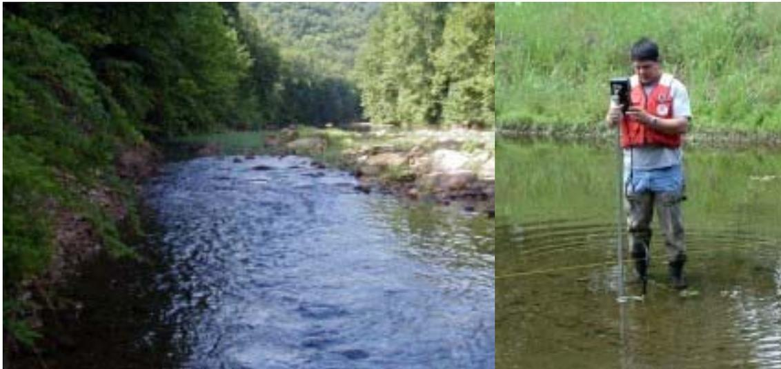
*Common stream-gauging conditions in Arkansas. The FlowTracker's integrated display and processor let you easily compute streamflow on the fly.*
