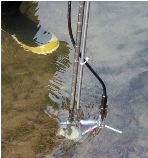
The probe is shown mounted to the wading rod. The unique 2D/3D design allows for 2D velocity measurements in water as shallow as one ft, or 3D measurements in 3D water.
