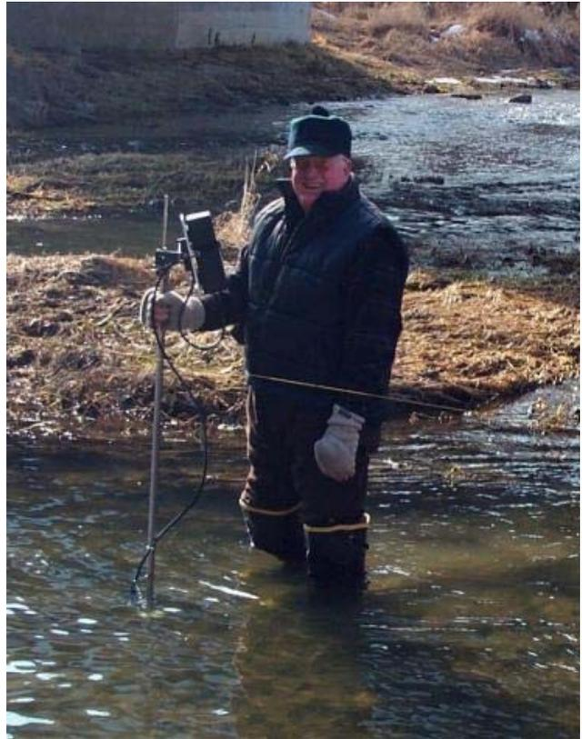
FlowTracker mounted on a top-setting wading rod
