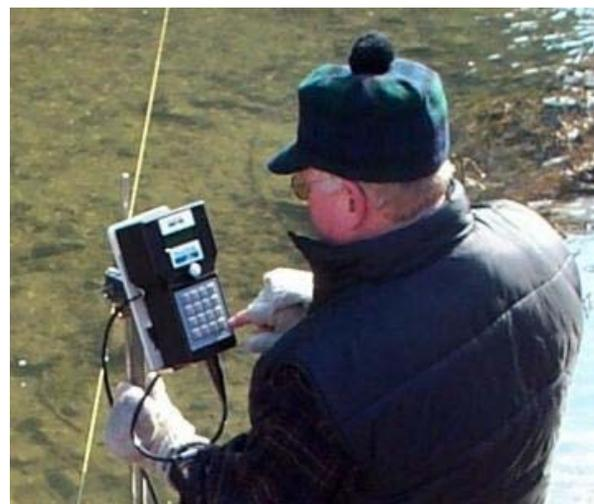
The integrated display and processor let you easily compute streamflow on-the-fly.
