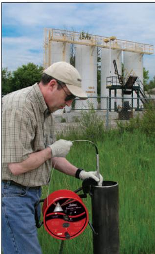
If the liquid is a non-conductive oil/product the signals are steady. If the liquid is water (conductive liquid greater than 20  $\mu\text{S}/\text{cm}$ ), the conductivity of the water completes a conductivity circuit. This overrides the infra-red circuit, and the tone and light are intermittent.
