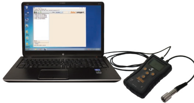
Figure 7-2 SRU to PC Connection
