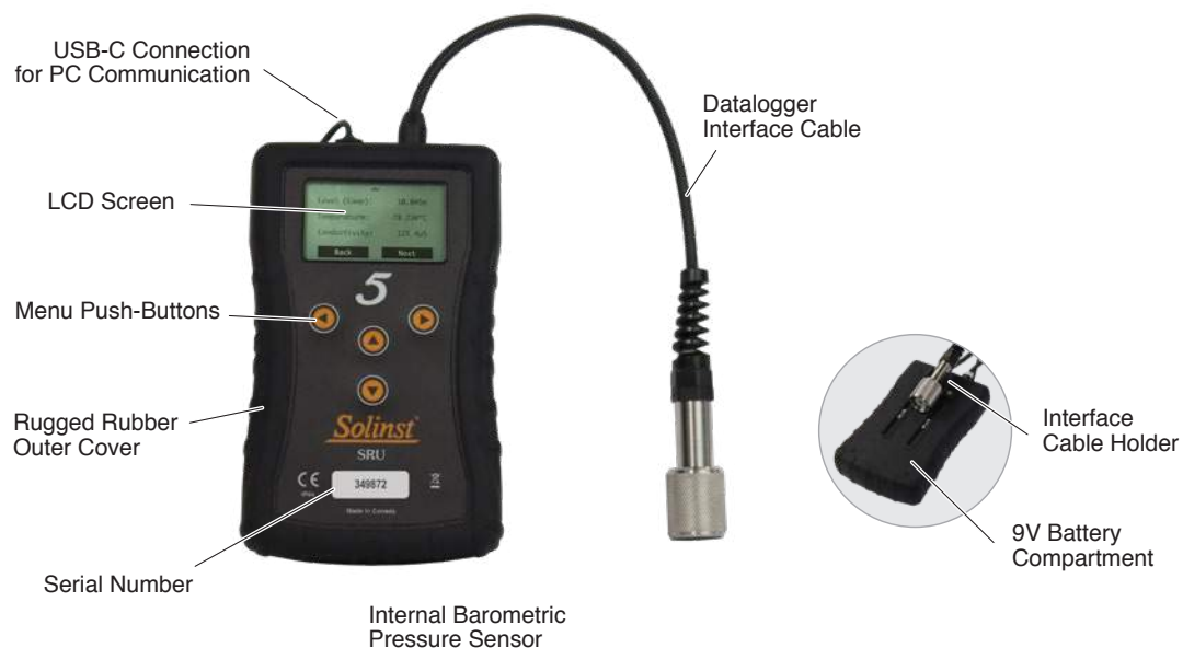
Figure 1-1 Solinst Readout Unit (SRU)
