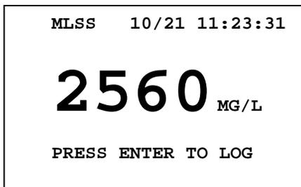
The analyzer and sensor have been zero calibrated at the factory and given a default span. In most cases, the factory default span will read reasonable values, but a span value based upon lab analysis should be performed as soon as possible. Span calibration can be accomplished using the snapshot/span feature described later in this manual. Separate span values for MLSS and RASS samples are available to insure maximum accuracy throughout the plant.
